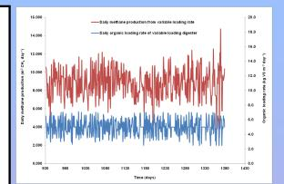
Fluctuations in gas production in response to random changes in loading between 2.5 -7.0 kg VS m<sup>3</sup> day<sup>-1</sup>
