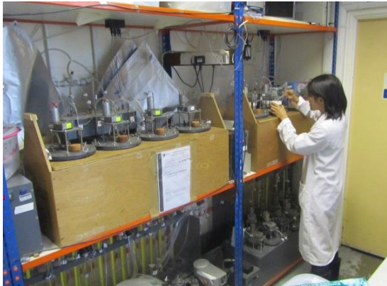
Continuously operated lab-scale digesters at Soton
