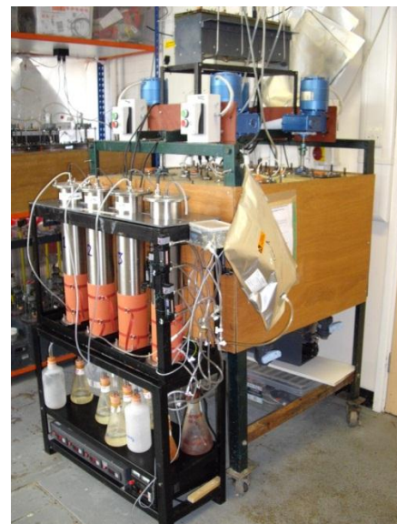
35-litre digesters and stripping columns
