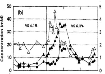
Changes in acetate ( $\Delta$ ) and propionate ( $\pm$ ) concentrations and P/A ratio ( $\bullet$ ) after a change in the HRT (left) and organic loading (right) (from Ahring et al., Appl Microbiol Biotechnol 43(1995), 559)
