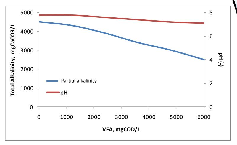
pH versus partial alkalinity for increasing VFA concentrations in the AD reactor
