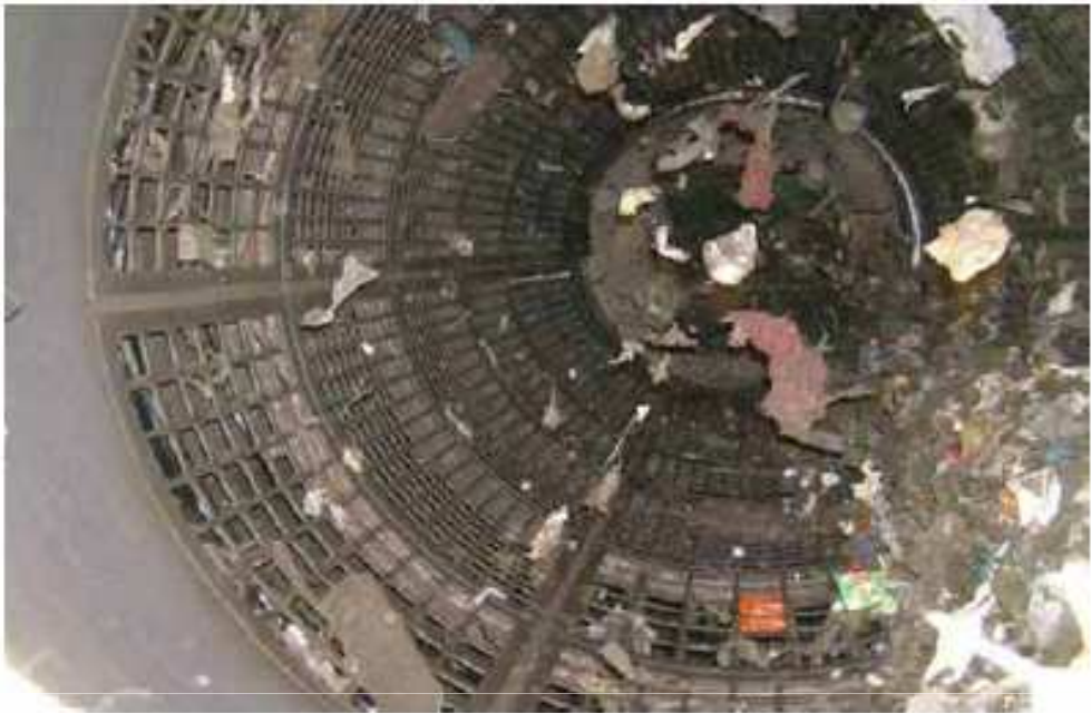
Figure 2: Waste separation using a trommel screen
