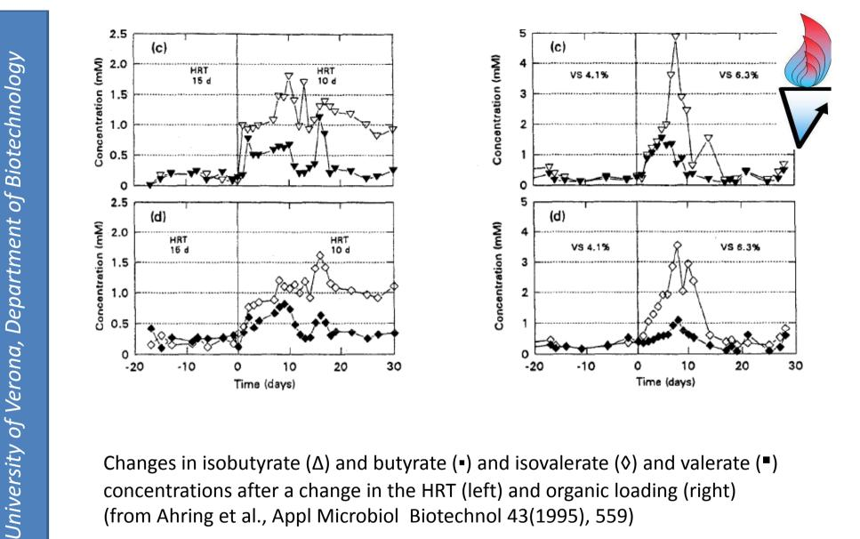
Changes in isobutyrate ( $\Delta$ ) and butyrate ( $\bullet$ ) and isovalerate ( $\diamond$ ) and valerate ( $\bullet$ ) concentrations after a change in the HRT (left) and organic loading (right) (from Ahring et al., Appl Microbiol Biotechnol 43(1995), 559)
