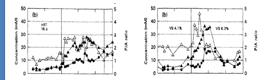
Changes in acetate ( $\Delta$ ) and propionate ( $\bigstar$ ) concentrations and P/A ratio ( $\bullet$ ) after a change in the HRT (left) and organic loading (right) (from Ahring et al., Appl Microbiol Biotechnol 43(1995), 559)
