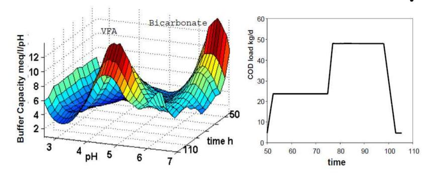
Figure 1: Buffers evolution from bicarbonate alkalinity to VFA during overload Figure 2: Organic overload to the reactor
