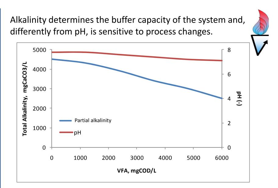
pH versus partial alkalinity for increasing VFA concentrations in the AD reactor
