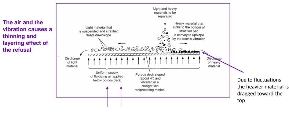
The blown-in air suspension keeps the lighter material being dragged down
