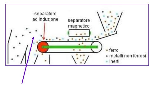
The metal components exposed to a magnetic field at high frequencies, are crossed by currents of Foucault that create a magnetic field.
