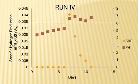
With  $\alpha = 1$ , pH system remained in range between 6.7 and 7 after seven days. In correspondence of these conditions, was not observed hydrogen production, instead was observed a small production of methane.
