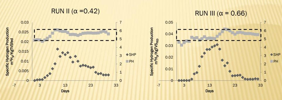
The trend of the hydrogen production, expressed as specific hydrogen production (SHP), in both of these runs, showed an initial low hydrogen production, due to the lag time, then a fast increase until a maximum value; after few days the production decreased though pH remains in the range of the functionality.
