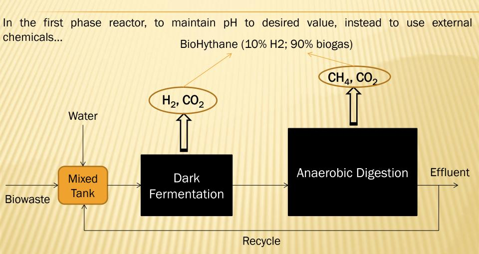
With this system, the production of hydrogen by DF of biowaste is obtained without external pH control because the recirculated second phase sludge supports the DF with buffering agents (mainly ammonia)
