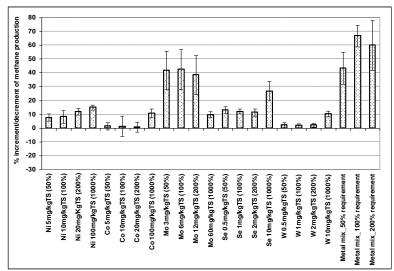
Figure 3. Histogram of increment or decrement on methane production of different condition tested compared to control test, expressed as a percentage. Results referred to Inoculum B
