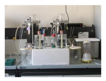
Figure 1: CSTR experimental apparatus.
