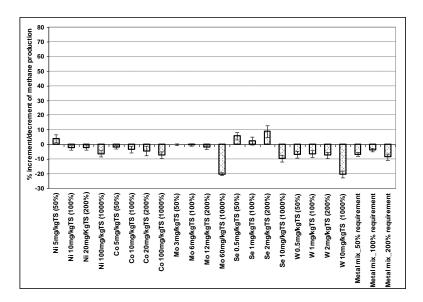
Figure 2: Histogram of increment or decrement on methane production of different condition tested compared to control test, expressed as a percentage. Results referred to Inoculum A
