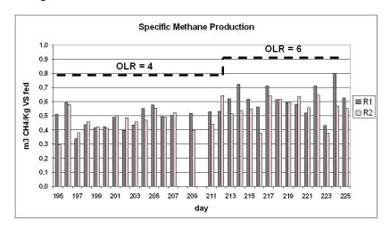
Figure 4. Comparison between Specific Methane Production of Reactor 1 and Reactor 2 during changing of OLR from 4 to 6.
