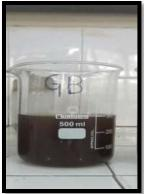
Water Obtained **Gunny Bag Filtration Set-Up** (~50 %) **Properties of removed water** EC: 5.83mS/cm , pH: 8.6, NTU: 812
