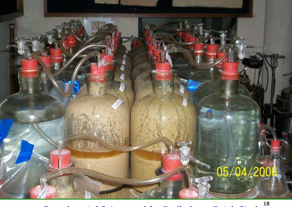
**Experimental Setup used for Preliminary Batch Study**
