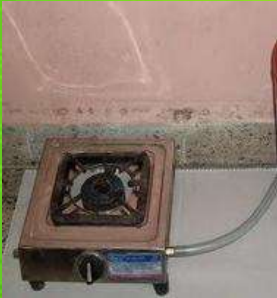
Upgraded and bottled biogas for use as a cooking fuel
