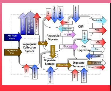
Energy inputs and outputs in the anaerobic digestion of source segregated food waste
