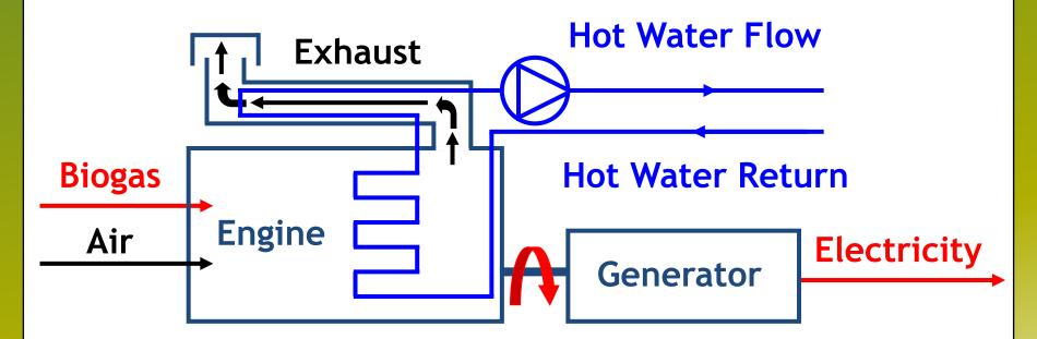
Biogas is piped to an engine which is either spark-ignition or dual fuel (with a fuel oil pilot). Heat is recovered from the engine jacket, the oil cooler and from the exhaust gas. Electricity conversion efficiencies vary from 25% to 42%, and 43% to 60% of the energy value of the biogas is converted to heat.
