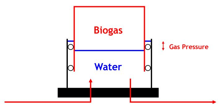
The gas bell floats on a tank of water guided by rollers. The gas pressure is determined by the weight of the bell and the internal area. The difference between the water level inside & outside is equal to the gas pressure.
