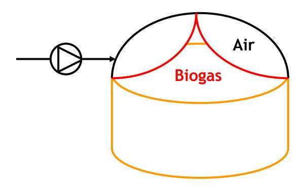
A very common digester design is to combine a double-membrane gas holder with the digester roof.
