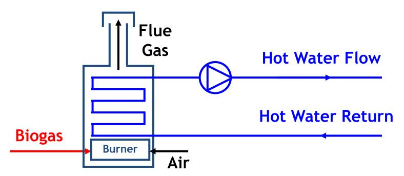
Gas boilers may be either atmospheric or pressurised burner type. Hot water is produced at an efficiency of about 85% with the rest of the energy as radiant heat and flue heat.
