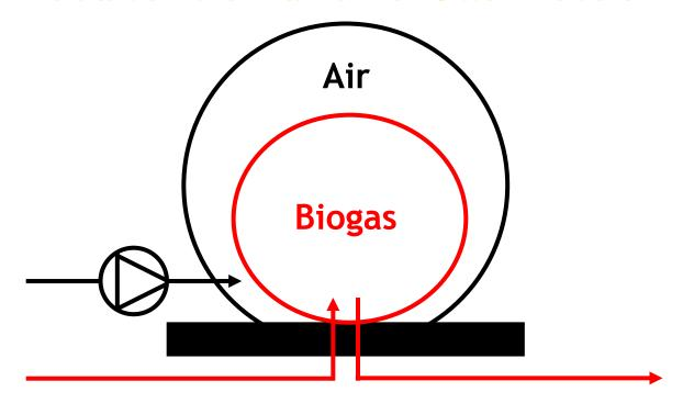
The air space between the two membranes is kept under a pressure of 100 to 200 mm water gauge by an air blower. The inner membrane expands and contracts under constant pressure to allow for variations in gas production and gas utilisation.
