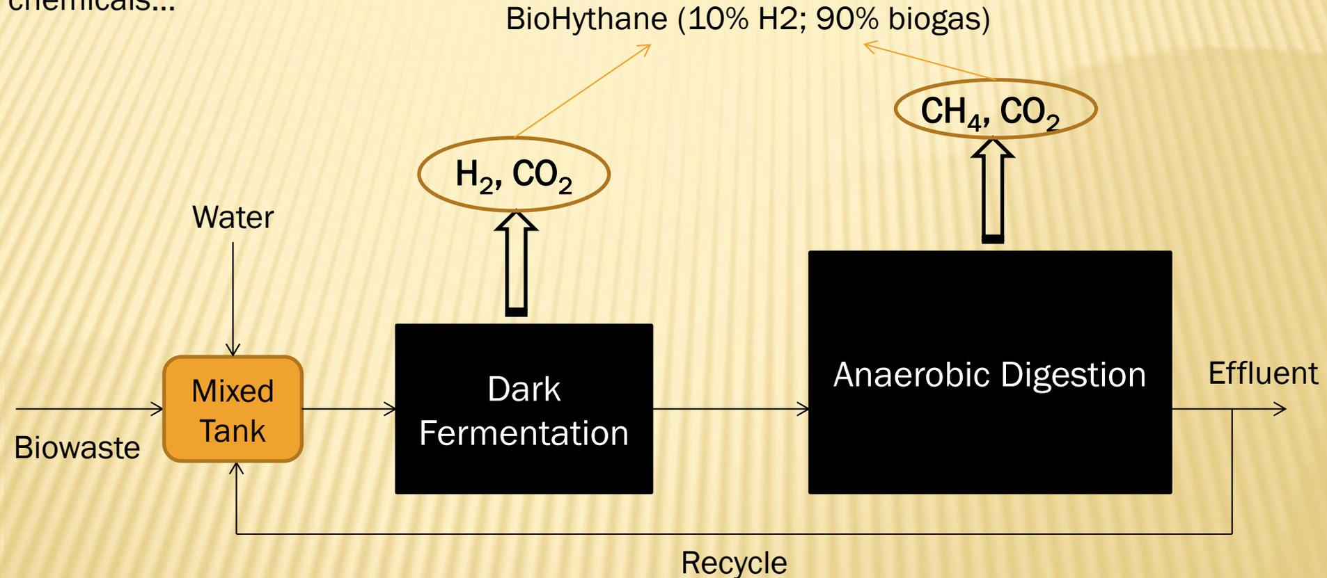
With this system, the production of hydrogen by DF of biowaste is obtained without external pH control because the recirculated second phase sludge supports the DF with buffering agents (mainly ammonia)
