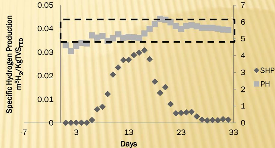
The trend of the hydrogen production, expressed as specific hydrogen production (SHP), in both of these runs, showed an initial low hydrogen production, due to the lag time, then a fast increase until a maximum value; after few days the production decreased though pH remains in the range of the functionality.
