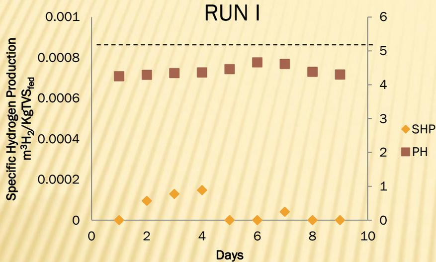
With  $\alpha = 0.33$ , pH maintained in range between 4.2 and 4.6. This low pH value could be explained by the low alkalinity in the system (stabilized at 800 mgCaCO<sub>3</sub>/L). This value of alkalinity was not sufficient to buffer the acids produced from fermentative process.
