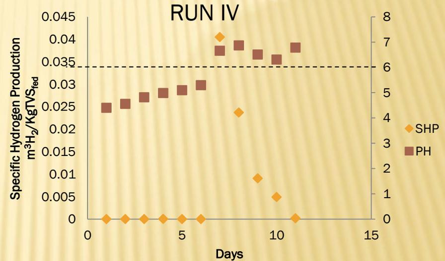
With  $\alpha = 1$ , pH system remained in range between 6.7 and 7 after seven days. In correspondence of these conditions, was not observed hydrogen production, instead was observed a small production of methane.
