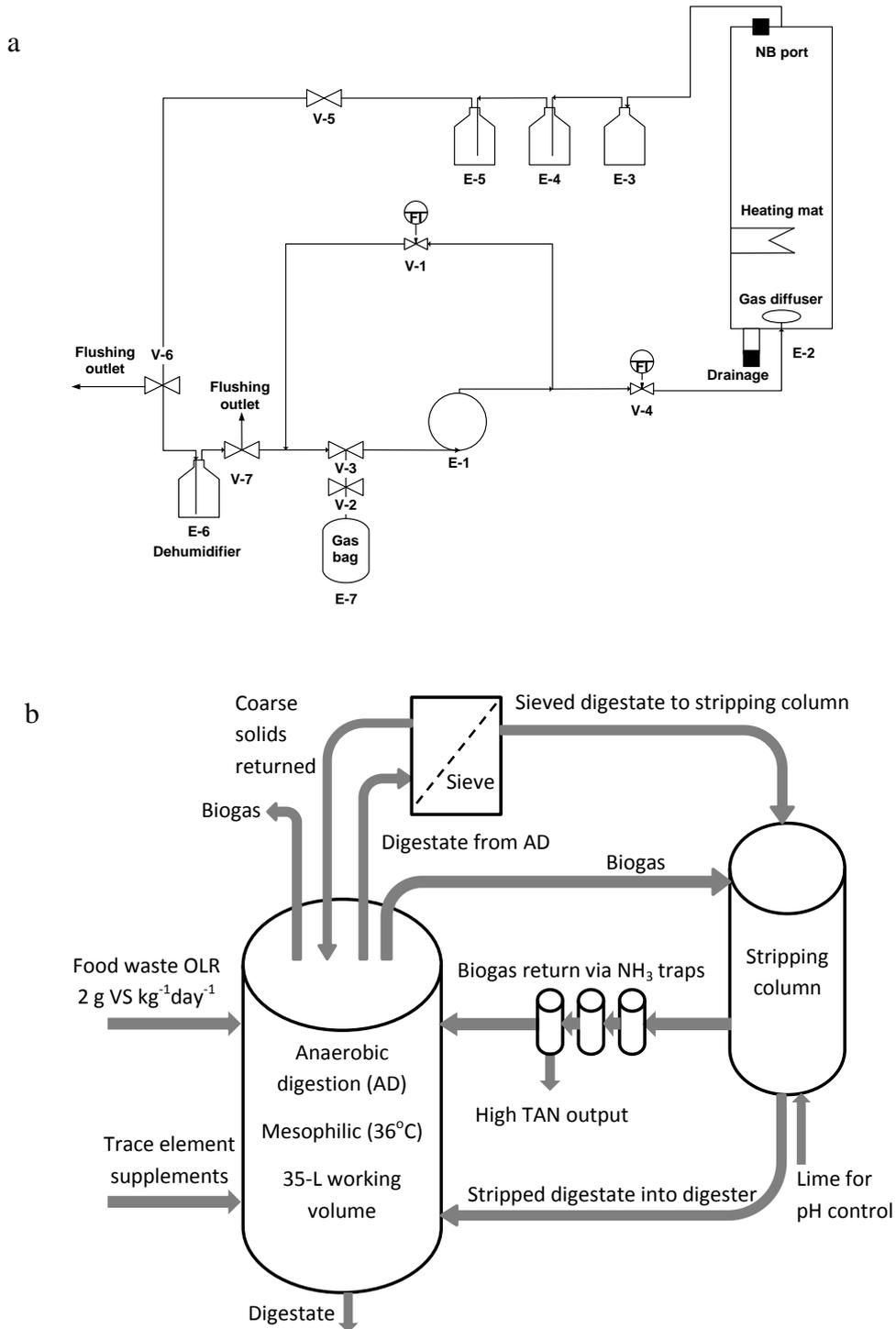
**Figure 1.** Details of experimental set-up (a) Process flow diagram for stripping column. E-1 diaphragm pump, E-2 stripping column, E-3 condensate trap, E-4 water trap, E-5 0.25N H<sub>2</sub>SO<sub>4</sub> trap, E-6 dehumidifier, E-7 gas bag; (b) Schematic of the coupled process.
