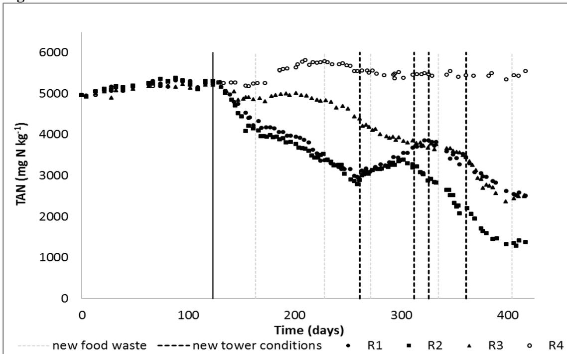
**Figure 2.** Total ammonia nitrogen in digestate during the experimental period. R<sub>1</sub>: closed circle. R<sub>2</sub>: closed square. R<sub>3</sub>: closed triangle. R<sub>4</sub>: open circle. Black continuous vertical line indicates start of stripping. Black discontinuous vertical lines indicate a change in stripping conditions (Table 2). Grey discontinuous vertical lines indicate a new batch of food waste (Table 1).
