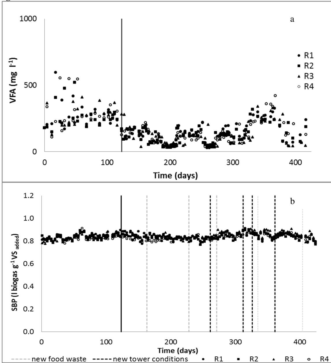
**Figure 3.** Total volatile fatty acid concentrations (a) and specific biogas production (b) during the experimental period. R<sub>1</sub>: closed circle. R<sub>2</sub>: closed square. R<sub>3</sub>: closed triangle. R<sub>4</sub>: open circle. Black continuous vertical line indicates start of stripping. Black discontinuous vertical lines indicate a change in stripping conditions (Table 2). Grey discontinuous vertical lines indicate a new batch of food waste (Table 1).
