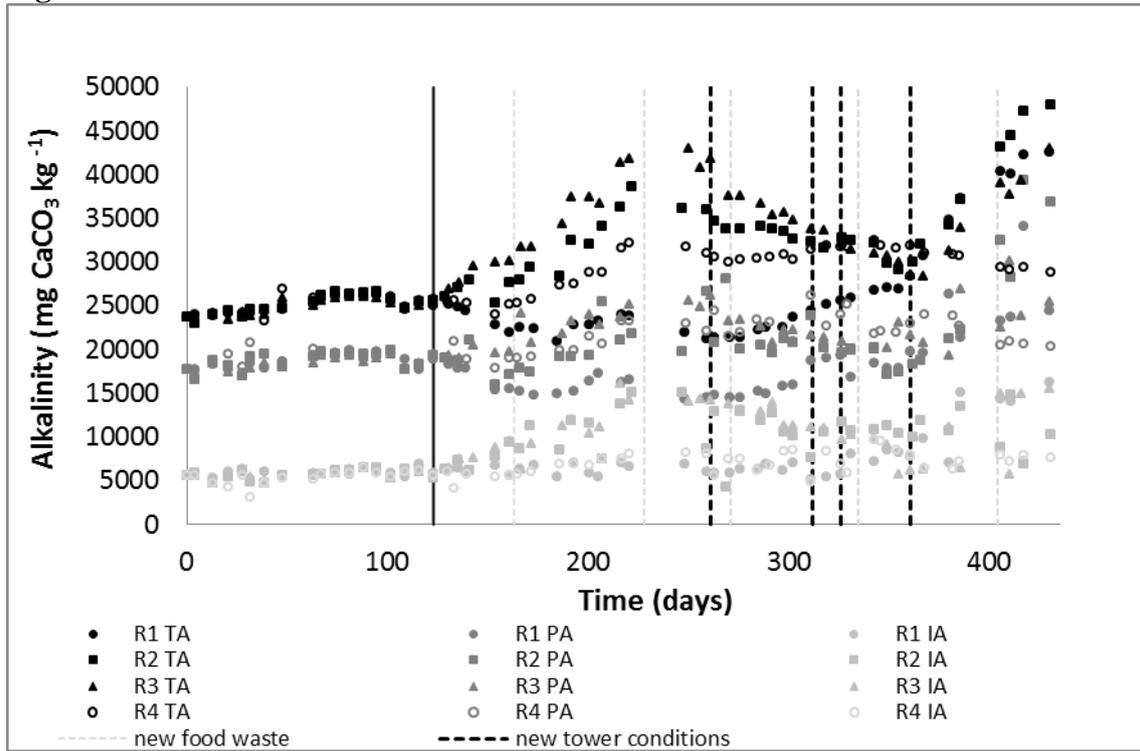
**Figure 4.** TA, PA and IA of digestate during the experimental period (black: TA, grey: PA, light-grey: IA). R<sub>1</sub>: closed circle. R<sub>2</sub>: closed square. R<sub>3</sub>: closed triangle. R<sub>4</sub>: open circle. Black continuous vertical line indicates start of stripping. Black discontinuous vertical lines indicate a change in stripping conditions (Table 2). Grey discontinuous vertical lines indicate a new batch of food waste (Table 1).
