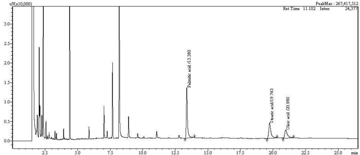
b) Chromatogram of identified LCFA from a digestate sample
