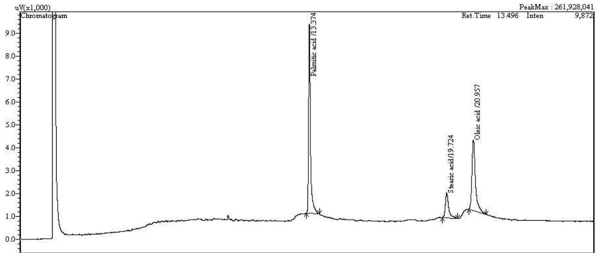
a) Representative chromatogram using a 50 mg l<sup>-1</sup> standard LCFA mix
