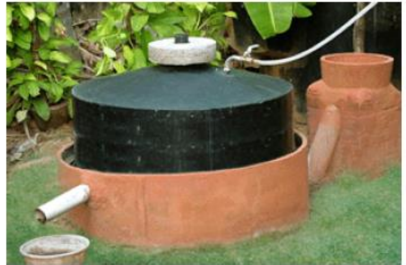
Picture 20: BIOTECH plant treating organic solid waste on a domestic level.
